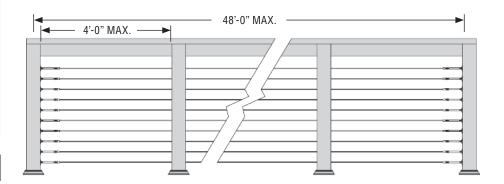
For straight cable sections using the RailEasy™ Tensioner at each end, you may run cable up to 48 feet in total length (mid post required as specified).
